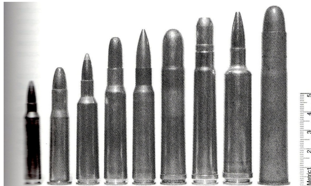
Figure 5 Various rifle bullets compared. Left to right: .223 caliber FMJ (M-16 assault rifle), 30-30 soft point, 6-mm soft point, 30-06 soft point, .308 caliber military-style FMJ (7.62 mm NATO), .458 caliber FMJ magnum, .375 caliber FMJ magnum, .378 caliber FMJ hollow tip, World War II-era .47 caliber FMJ. FMJ, full metal jacket. (Bullets courtesy of Bruce Ham, MD, and Gerald Warnock, MD, Portland, OR.)
